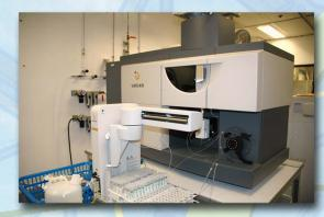
This high sample throughput ICP-OES is capable of measuring concentrations of multi-metals at ppm level. The Auto-sampler can handle as many as 180 samples. For determination of certain elements whose sensitivity is lower (e.g. mercury), the optional Vapor Generation Accessory (VGA) can be equipped to enhance the sensitivity while the detection limit can be lowered to ppb level.
