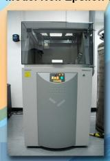
EDXRF is used to determine elemental composition of aerosol filter samples, thin film, soil, metal, oil, and liquid (non-volatile) samples. It can detect elements in the periodic
