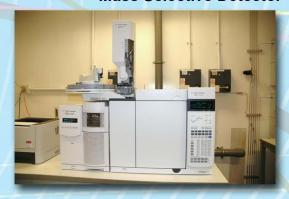
The GC-MSD is composed of a split/splitless capillary injector, an automatic liquid sampler and a single quadrupole mass spectrometer that can cover the mass up to 1050 Da. It can separate and quantitatively measure organic compounds that are volatile enough to be vaporized without decomposition in the split/splitless injector. MSD can produce a 3D data set (both chromatogram and mass spectra at the same time) for better understanding of the components in a sample.
