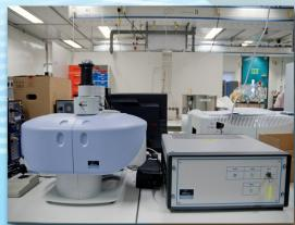
This RAMAN Microscope can generate Raman spectrum, ranging from 3500 to 95 cm<sup>-1</sup> and with resolution down to 1 cm<sup>-1</sup> to aid qualitative analysis of solid samples. It is used in many varied applications including pharmaceuticals, polymer study, printing and chemical analysis.
