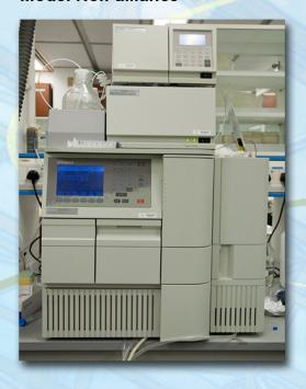
The instrument provides separation and qualitative/quantitative determination of samples and is widely applied in environmental, pharmaceutical, and biochemical analysis.
