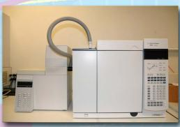
The GC-ECD can separate and quantitatively measure organic compounds that are volatile enough to be vaporized without decomposition in the Headspace 7890A system (ambient to 200 °C). The ECD installed in the GC is sensitive towards organic molecules that contain halogen, peroxides, quinones and nitro functional groups. Molecules with double bond can also be determined but with less sensitivity.
