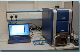
The table top Scanning Electron Microscope (SEM) can magnify an object from 50 to 30,000 times. The microscope can be used for image recording, qualitative elemental analysis and morphological investigations of specimen including biological sample, print circuit board, particles, etc. In addition, a Silicone Drift Detector (SDD) is installed in the microscope for elemental composition analysis. Elements from Boron to Americium can be detected and mapped on the specimen image.
